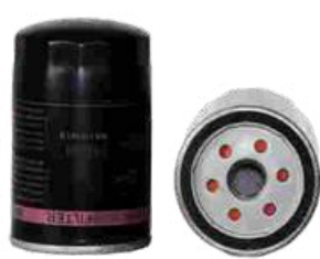
FXO-ALO-008 Largest OD: Φ76(mm) Overall Height: 126(mm) Thread Size: 3/4-16UNF
