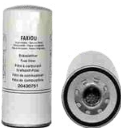
FXO-CF-020 Largest OD: 108(mm) Overall Height: 260(mm) Thread Size: M32X1.5 OEM: 20430751FUEL: 20430751 VOLVO: 20405160,20976003, 20815011,20430751 RENAULT: 7420976001, 7420541381 MANN: 51.125.030.053, WDK11102/11 FLEETGUARD: FF5507 HENGST: H200WDK
