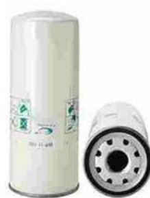
FXO-BO-007 Largest OD: 108(mm) Overall Height: 260(mm) Thread Size: 1 3/8"-16
