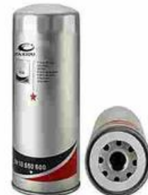
FXO-LO-009 Largest OD: 108(mm) Overall Height: 260(mm) Thread Size: 1 1/8"-16
