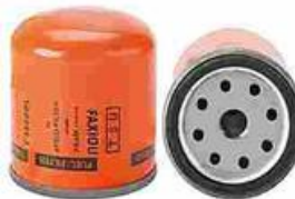
FXO-AFF-001 Largest OD: 77(mm) Overall Height: 80(mm) Thread Size: M16X1.5
