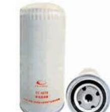
FXO-DF-044 Largest OD: 95(mm) Overall Height: 208(mm) Thread Size: M16X1.5 OEM: FF4070 FLEETGUARD: FF4070
