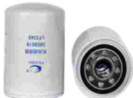
FXO-DO-027 Largest OD: 94(mm) Overall Height: 135(mm) Thread Size: 1"-16UNF
