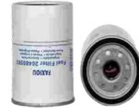
FXO-CF-011 Largest OD: 94(mm) Overall Height: 138.5(mm) Thread Size: 1"-14UNF OEM: 20480593 VOLVO: 20998346,20514654 20480593,20998367RENAULT: 7420514654, 7420541383,7420998634 MANN: WK940/33X FLEETGUARD: FS19735 HENGST: H700WK
