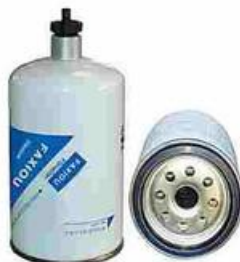
FXO-HF-046 Largest OD: 108(mm) Overall Height: 210(mm) Thread Size: 1"-14UNF OEM: R60-10-HP
