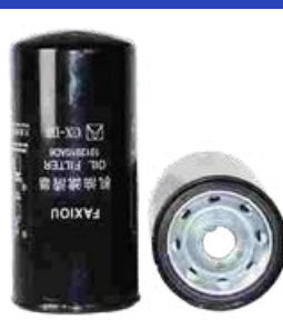
FXO-AKO-004 Largest OD: Φ108(mm) Overall Height: 232.5(mm) Thread Size: 11/8"-16
