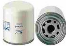
FXO-GO-004 Largest OD: 95(mm) Overall Height: 113(mm) Thread Size: M23X1.5
