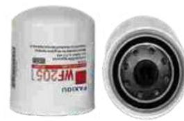
FXO-DC-002 Largest OD: 94(mm) Overall Height: 105(mm) Thread Size: 11/16"-16 OEM: WF2051 HENGST: H13WF12 CAT: 9N-3368 CUMMINS: 259453 DAF: 13692 KOMATSU: 381-625-6271 NISSAN: 21915-95000 RENAULT: 5000 808721 VOLVO: 200973329
