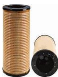
FXO-AO-023 Largest OD: 130(mm) Overall Height: 280(mm) Thread Size: Φ85,Φ85 OEM: 1R-0774 PU芯 CAT: 1R-0774 FLEETGUARD: HF6202
