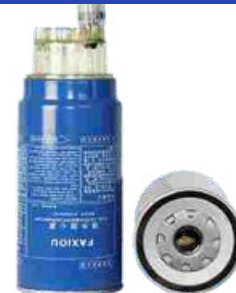
FXO-AHF-002 Largest OD: 108(mm) Overall Height: 319(mm) Thread Size: 1"-14UNF
