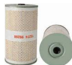
FXO-YO-005 Largest OD: 130(mm) Overall Height: 243(mm) Thread Size: Φ28,Φ28 OEM: 1527499288 NISSAN: 1527499288 FLEETGUARD: LF3629
