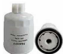
FXO-DF-052 Largest OD: 78(mm) Overall Height: 113(mm) Thread Size: M16X1.5
