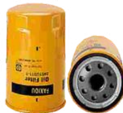
FXO-AO-005 Largest OD: 108(mm) Overall Height: 160(mm) Thread Size: 1 1/8"-16 OEM: 2451U311-1 KOBELCO: 2451U311-1
