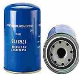
FXO-JF-003 Largest OD: 94(mm) Overall Height: 145(mm) Thread Size: M24X1.5
