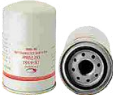
FXO-AO-013 Largest OD: 94(mm) Overall Height: 138(mm) Thread Size: 1 1/8"-16 OEM: 8N-9586 CAT: 8N-9586, 1N-3224,1R-0713 HINO: 349261040 KOMATSU: 3ED-661-1330 RENAULT: 5000816061 VOLVO: 11939676
