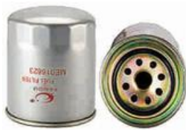
FXO-XF-003 Largest OD: 80(mm) Overall Height: 100(mm) Thread Size: M20X1.5 OEM: ME016823 MITSUBISHI: 055923570, ME016823 BF825F
