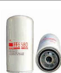
FXO-DF-047 Largest OD: 94(mm) Overall Height: 170(mm) Thread Size: 7/8"-14 OEM: FF5580 FLEETGUARD: FF5078 PERKINS: 26560137 P26562003
