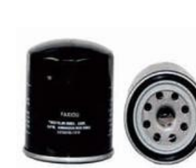
FXO-WO-007 Largest OD: 89(mm) Overall Height: 100(mm) Thread Size: M20X1.5
