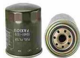
FXO-SF-013 Largest OD: 102(mm) Overall Height:125 (mm) Thread Size: 1"-14
