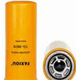
FXO-AO-020 Largest OD: 95(mm) Overall Height: 248(mm) Thread Size: 1 3/8"-12 OEM: 1G- 8878CAT: 1G-8878 HENGST: H18W11 VOLVO: 11036607-7 FLEETGUARD: HF6553 MANN: WH980/3 JOHNDEERE: RE47313 DONALDSON: P177047
