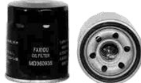
FXO-XO-003 Largest OD: 67(mm) Overall Height: 87(mm) Thread Size: M20X1.5
