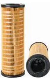
FXO-AO-021 Largest OD: 78.5(mm) Overall Height:229 (mm) Thread Size: Φ47,Φ47 OEM: 1R-0728 CAT: 1R-0728 FLEETGUARD: LF6201
