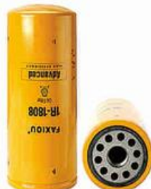
FXO-AO-018 Largest OD: 136(mm) Overall Height: 308(mm) Thread Size: 1 1/2"-16 OEM: 1R-1808 CAT: 1R-1808 FLEETGUARD: LF691A
