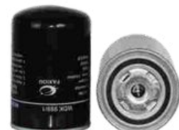
FXO-BF-022 Largest OD: 94(mm) Overall Height: 145(mm) Thread Size: M18X1.5
