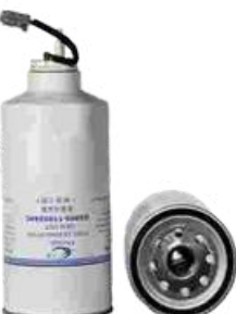
FXO-AIF-006 Largest OD: 108(mm) Overall Height: 287(mm) Thread Size: 1"-14UNF
