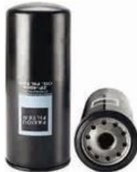
FXO-AO-015 Largest OD: 108(mm) Overall Height: 265(mm) Thread Size: 1 1/8"-16 OEM: 2P-4004 HENGST: H200W04 MANN: W11102/27 CAT: 1R-0658,1R-0739, 1W-3300,2P-4004
