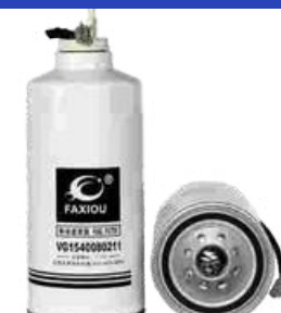
FXO-AKF-003 Largest OD: 108(mm) Overall Height: 240(mm) Thread Size: 1"-14UNF
