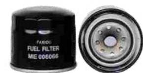
FXO-XF-001 Largest OD: 89(mm) Overall Height: 81(mm) Thread Size: M20X1.5 OEM: ME006066 MANN: WK818/80 CAT: 094-7073
