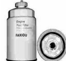
FXO-TF-004 Largest OD: 85(mm) Overall Height: 163(mm) Thread Size: M16X1.5
