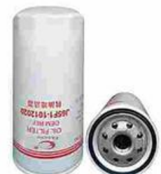
FXO-AIO-010 Largest OD: 110(mm) Overall Height: 210(mm) Thread Size: 1,1/8"-16
