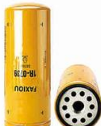
FXO-AO-019 Largest OD: 108(mm) Overall Height: 265(mm) Thread Size: 1 1/8"-16 OEM: 1R-0739 HENGST: H200W04 MANN: W11102/27 CAT: 1R-0658,1R-0658 RENAULT: 20709459 VOLVO: 478362
