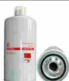
FXO-DF-036 Largest OD: 94(mm) Overall Height: 200(mm) Thread Size: 1"-14 OEM: 1119ZB6-030 FLEETGUARD: FF5078 PERKINS: 26560137 P26562003
