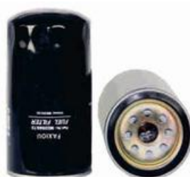
FXO-XF-005 Largest OD: 94(mm) Overall Height: 175(mm) Thread Size: M24X1.5 OEM: ME056670 HYUNDAI: KSH0457 MANN: 4326739 MITSUBISHI: ME056670
