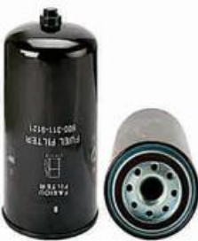
FXO-FF-017 Largest OD: 94(mm) Overall Height: 188(mm) Thread Size: 1"-14UNF
