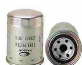
FXO-SF-003 Largest OD: 81(mm) Overall Height: 100.5(mm) Thread Size: 3/4"-16
