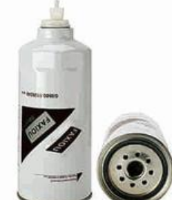
FXO-AIF-008 Largest OD: 108(mm) Overall Height: 240(mm) Thread Size: 1"-14UNF
