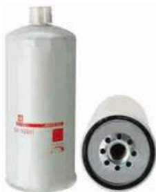
FXO-DF-029 Largest OD: 108(mm) Overall Height: 260(mm) Thread Size: 1"-14UNF OEM: F170 FLEETGUARD: FS19789,F170 11192D2A-030
