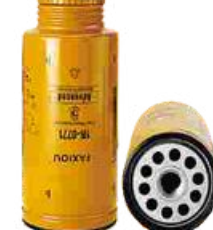
FXO-AF-020 Largest OD: 108(mm) Overall Height: 235(mm) Thread Size: 1"-14
