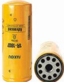
FXO-AO-012 Largest OD: 108(mm) Overall Height: 265(mm) Thread Size: 1 1/8"-16 OEM: 1R-1807 CAT: 1R-1807 FLEETGUARD: LF3379, LF3321, LF667, LF16101
