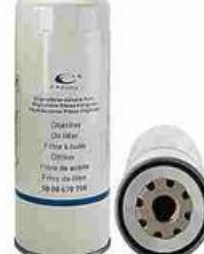
FXO-LO-006 Largest OD: 108(mm) Overall Height: 260(mm) Thread Size: 1 1/8"-16
