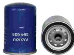
FXO-JF-002 Largest OD:77 (mm) Overall Height:118 (mm) Thread Size: M16×1.5
