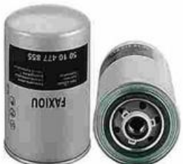
FXO-LF-003 Largest OD: 94(mm) Overall Height: 145(mm) Thread Size: M18X1.5
