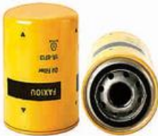
FXO-AO-001 Largest OD: 94(mm) Overall Height: 135(mm) Thread Size: 1 1/8"-16 OEM: 1R-0713 CAT: 1R-0713 FLEETGUARD: LF3342
