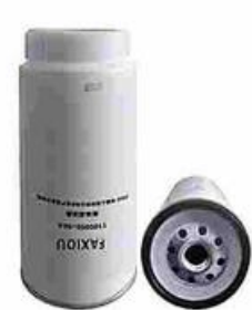
FXO-ALF-006 Largest OD: Φ108(mm) Overall Height: 228(mm) Thread Size: 1"-14
