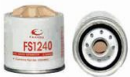
FXO-DF-025 Largest OD: 94(mm) Overall Height: 90(mm) Thread Size: M16X1.5 OEM: FS1240 FLEETGUARD: FS1240
