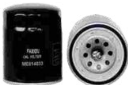
FXO-XO-001 Largest OD: 101(mm) Overall Height: 124(mm) Thread Size: M20X1.5
