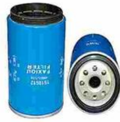
FXO-JF-004 Largest OD: 108(mm) Overall Height: 181(mm) Thread Size: 1"-14UNF
