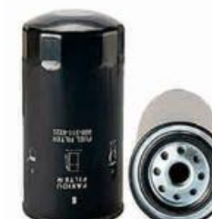
FXO-FF-011 Largest OD: 77(mm) Overall Height: 116(mm) Thread Size: 3/4"-16
