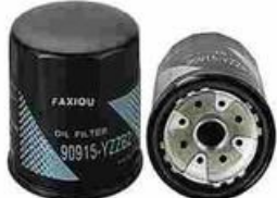
FXO-UO-005 Largest OD: 74(mm) Overall Height: 80(mm) Thread Size: 3/4"-16
