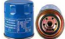
FXO-VO-003 Largest OD: 91(mm) Overall Height: 93(mm) Thread Size: M18X1.5
