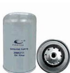
FXO-NO-008 Largest OD:108(mm) Overall Height:165 (mm) Thread Size: M16X1.5
