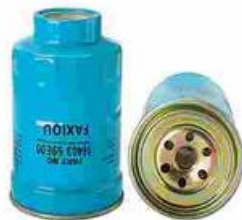
FXO-YF-005 Largest OD: 94(mm) Overall Height: 137(mm) Thread Size: 3/4"-16 M36X1.5
