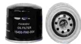
FXO-AAO-001 Largest OD: 90(mm) Overall Height: 80(mm) Thread Size: M22*1.5
