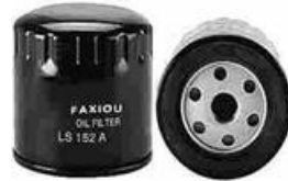
FXO-ABO-001 Largest OD: 85(mm) Overall Height: 89(mm) Thread Size: M18X1.5
