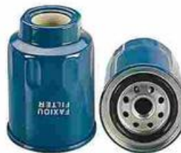
FXO-WF-008 Largest OD: 79(mm) Overall Height: 100(mm) Thread Size: 3/4"-16
