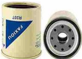
FXO-HF-027 Largest OD: 94(mm) Overall Height: 100(mm) Thread Size: 1"-14UNF OEM: R20T HENGST: H7020WK10 MANN: WK924/1X VOLVO: 857633
