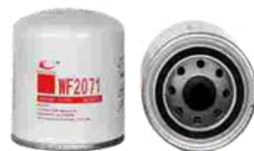
FXO-DC-005 Largest OD: 94(mm) Overall Height: 105(mm) Thread Size: 11/16"-16
