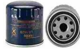
FXO-ABO-002 Largest OD: 85(mm) Overall Height: 89(mm) Thread Size: M18X1.5
