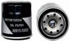
FXO-UO-001 Largest OD: 74(mm) Overall Height: 87(mm) Thread Size: 3/4"-16
