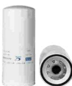
FXO-BO-008 Largest OD: 108(mm) Overall Height: 260(mm) Thread Size: 1 1/8"-16
