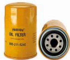
FXO-FO-014 Largest OD: 94(mm) Overall Height: 135(mm) Thread Size: 1"-12
