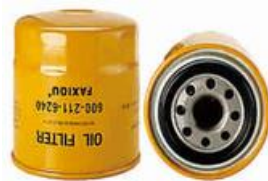
FXO-FO-013 Largest OD: 94(mm) Overall Height: 98(mm) Thread Size: 1"-12
