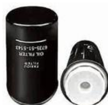
FXO-FO-018 Largest OD: 95(mm) Overall Height: 172(mm) Thread Size: 1"-16
