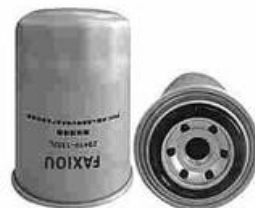
FXO-SF-016 Largest OD:85(mm) Overall Height: 103(mm) Thread Size: 3/4"-16
