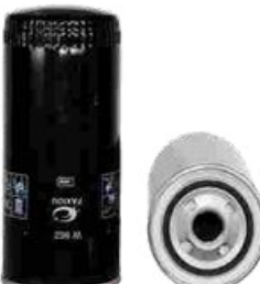
FXO-BO-012 Largest OD: 94(mm) Overall Height: 208(mm) Thread Size: 1"-12UNF OEM: W962MANN: W962 HENGST: H18W01 IVECO: 1160025 BENZ: 0011849601 RENAULT: 0024164103 VOLVO: 11993545-0 DEUTZ: 01174421
