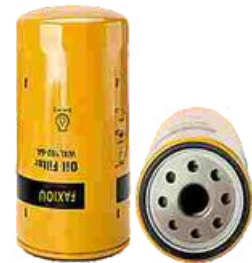
FXO-AO-009 Largest OD: 108(mm) Overall Height: 200(mm) Thread Size: 1 1/8"-16 OEM: 192-6A
