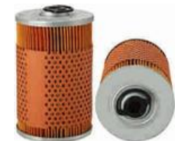
FXO-OTF-118 Largest OD: 84(mm) Overall Height: 145(mm) Thread Size: Φ13,Φ13 OEM: KX36 DEUTZ: 1168398 MANN: P811 HYUNDAI: 24749-026 ISUZU: 6-11070-620-1 IVECO: 1289054 KOMATSU: 611-070-6202
