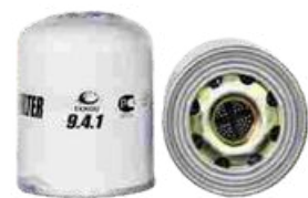
FXO-BA-001 Largest OD: 136(mm) Overall Height: 165(mm) Thread Size: M39X1.5
