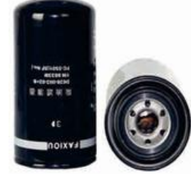
FXO-AJF-008 Largest OD: 94(mm) Overall Height: 173(mm) Thread Size: 1"-14UNF
