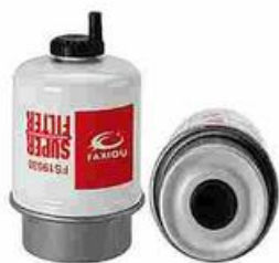
FXO-DF-026 Largest OD: 82(mm) Overall Height: 133(mm) Thread Size: M16X1.5 OEM: FS19530 HENGST: H183WK MANN: WK8122 CAT: 1006374 PERKINS: 2650920
