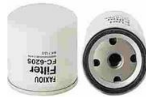
FXO-BF-001 Largest OD: 76(mm) Overall Height: 80(mm) Thread Size: M16X1.5
