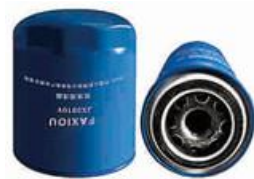
FXO-AIO-001 Largest OD: 94(mm) Overall Height: 100(mm) Thread Size: M24X2
