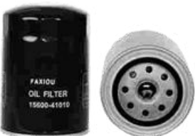
FXO-UO-009 Largest OD: 92(mm) Overall Height: 135 (mm) Thread Size: 3/4"-16
