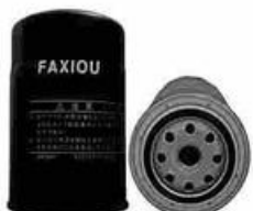
FXO-UO-010 Largest OD: Φ98(mm) Overall Height: 140(mm) Thread Size: 3/4"-16
