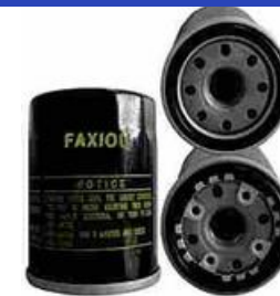
FXO-UO-014 Largest OD: Φ68(mm) Overall Height: 84(mm) Thread Size: 3/4"-16 OEM: 90915-10002
