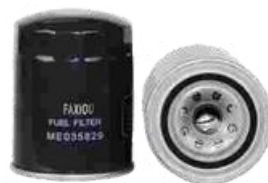
FXO-XF-002 Largest OD: 89(mm) Overall Height: 120 (mm) Thread Size: M20*1.5 OEM: ME035829 MITSUBISHI: ME035393
