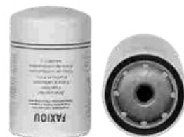
FXO-CF-016 Largest OD: 77(mm) Overall Height: 120(mm) Thread Size: M16X1.5
