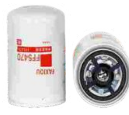
FXO-DF-037 Largest OD: 92(mm) Overall Height: 145(mm) Thread Size: M18X1.5 OEM: FF5470
