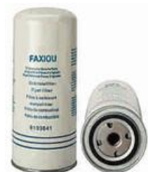
FXO-CF-018 Largest OD: 94(mm) Overall Height: 210(mm) Thread Size: M18×1.5
