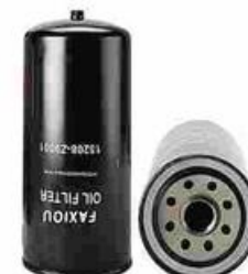
FXO-YO-004 Largest OD: 108(mm) Overall Height: 220(mm) Thread Size: 1 1/8"-16 OEM: 15208-Z9001 NISSAN: 15208-Z9001 FLEETGUARD: LF3436
