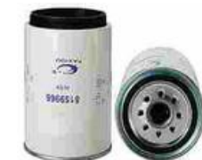
FXO-CF-017 Largest OD: 108(mm) Overall Height: 155(mm) Thread Size: 1"-14UNF
