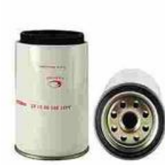
FXO-EF-001 Largest OD: 108(mm) Overall Height: 155(mm) Thread Size: 1"-12UNF
