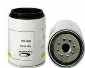
FXO-SF-008 Largest OD: 108(mm) Overall Height: 126(mm) Thread Size: 1"-14UNF
