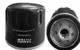
FXO-LO-002 Largest OD: 77(mm) Overall Height: 64(mm) Thread Size: M20X1.5
