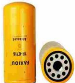
FXO-AO-011 Largest OD: 136(mm) Overall Height: 308(mm) Thread Size: 1 1/2"-16 OEM: 1R-0716 CAT: 1R-0716 FLEETGUARD: LF691
