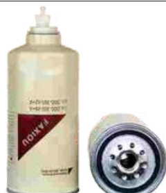
FXO-HF-034 Largest OD: 108(mm) Overall Height: 242(mm) Thread Size: 1"-14UNF OEM: D00-305-02+A VG1540080211,G5800-1105240
