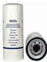
FXO-CO-006 Largest OD: 108(mm) Overall Height: 260(mm) Thread Size: 1 1/8"-16
