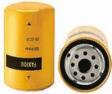
FXO-AO-004 Largest OD: 94(mm) Overall Height: 135(mm) Thread Size: 1"-12 OEM: 1R-0734 CAT: 1R-0734 FLEETGUARD: LF654 KOMATSU: 600-211-5240
