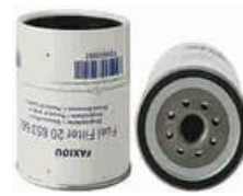
FXO-CF-001 Largest OD: 108(mm) Overall Height: 124(mm) Thread Size: 1"-14UNF
