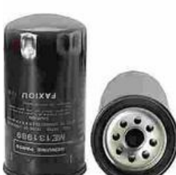
FXO-XF-007 Largest OD: (mm) Overall Height: 172(mm) Thread Size: M24X1.5 OEM: ME131989 MITSUBISHI: ME131989 ME056280
