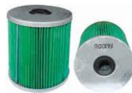
FXO-XF-012 Largest OD: 92(mm) Overall Height: 117(mm) Thread Size: Φ20,Φ20 OEM: ME036478 ME036116
