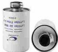
FXO-CA-003 Largest OD: 88(mm) Overall Height: 133(mm) Thread Size: Φ29
