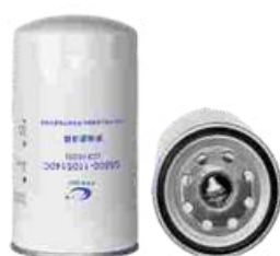
FXO-AIF-002 Largest OD: 108(mm) Overall Height: 200(mm) Thread Size: 1"-14UNF
