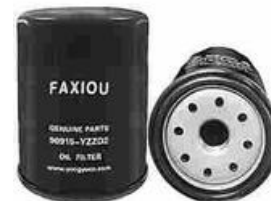
FXO-UO-017 Largest OD: Φ77.5(mm) Overall Height: 88(mm) Thread Size: 3/4"-16
