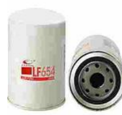
FXO-DO-014 Largest OD: 94(mm) Overall Height: 137(mm) Thread Size: 1"-12 OEM: LF654 HENGST: H17W04 CUMMINS: 851220031 DAF: 690260 DEUTZ: 0150-15-75.10 KOMATSU: 600-211-5240
