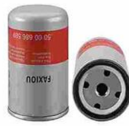
FXO-LF-005 Largest OD: 77(mm) Overall Height: 120(mm) Thread Size: M16X1.5
