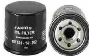
FXO-ZO-001 Largest OD: 68(mm) Overall Height: 67.3(mm) Thread Size: M20X1.5
