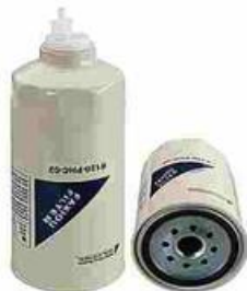
FXO-HF-032 Largest OD: 108(mm) Overall Height: 288(mm) Thread Size: 1"-14UNF OEM: R120-PHC-02 PK: R120-PHC-02, VG1540080211
