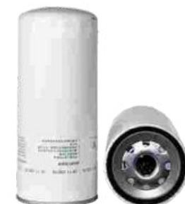
FXO-BO-006 Largest OD: 108(mm) Overall Height: 260(mm) Thread Size: 1,1/8"-16
