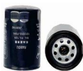
FXO-ALF-011 Largest OD: Φ94(mm) Overall Height:135(mm) Thread Size: 1"-16
