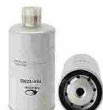
FXO-IF-008 Largest OD: 82(mm) Overall Height: 130(mm) Thread Size: M16X1.5
