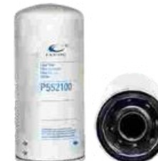
FXO-KC-002 Largest OD: 118(mm) Overall Height: 256 (mm) Thread Size: 1 1/2", 5/8"-12 OEM: P552100
