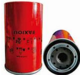
FXO-OF-004 Largest OD: Φ96.5(mm) Overall Height: 143(mm) Thread Size: 1"-14
