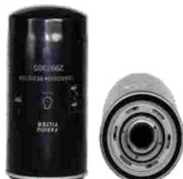
FXO-NO-007 Largest OD: 108(mm) Overall Height: 213(mm) Thread Size: M30X2
