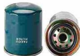
FXO-WF-006 Largest OD: 79(mm) Overall Height: 88(mm) Thread Size: 3/4"-16
