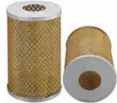
FXO-OTF-110 Largest OD: 72.5(mm) Overall Height: 113(mm) Thread Size: Φ24,Φ24 OEM: CHA100X150-BA
