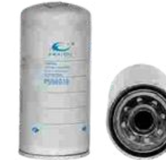
FXO-KC-003 Largest OD: 97(mm) Overall Height: 202(mm) Thread Size: 1-12
