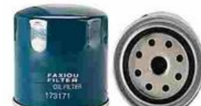
FXO-JOF-X000-50-003 Largest OD: 95(mm) Overall Height: 90(mm) Thread Size: 3/4"-16
