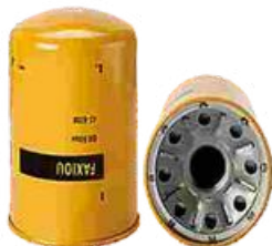
FXO-AO-006 Largest OD: 129(mm) Overall Height: 170(mm) Thread Size: 1 1/2"-16 OEM: 4I-6788 CAT: 4I-6788 FLEETGUARD: HF6710
