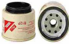
FXO-HF-037 Largest OD: 77(mm) Overall Height: 65(mm) Thread Size: M18X1.5 OEM: R12P RACOR: R12P FLEETGUARD: FS19627
