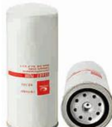
FXO-DC-012 Largest OD: 94(mm) Overall Height: 190(mm) Thread Size: 11/16"-16
